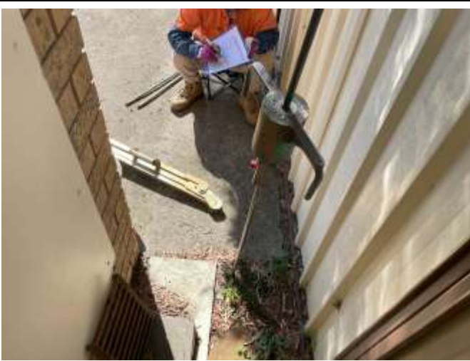
Photograph 1 Dynamic Cone Penetrometer(DCP) Test in progress at location of DCP1 within rear portion
