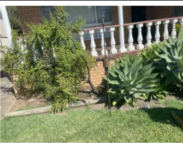
Photograph 2 DCP test in progress at location of DCP2 within front portion
