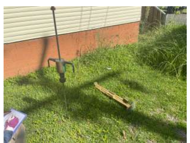
Photograph 4 DCP test in progress at DCP3 within front yard
