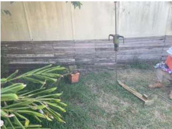
Photograph 3 DCP test in progress at DCP3 within rear portion portion
